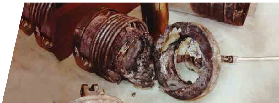
Image of the charred remains of the lithium perchlorate canister returned from space station Mir.
